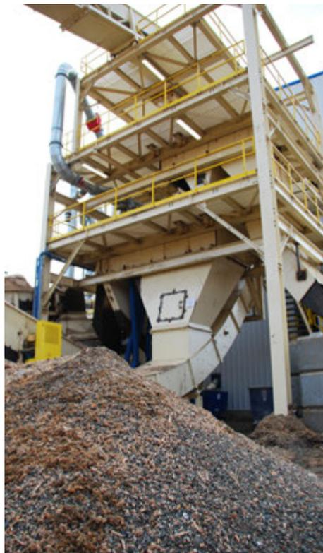
The entire ClassiCleaner system is housed in three separate towers connected by a series of conveyors.
